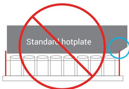
3. Raised perimeter rim and the rim is taller than the chimneys.
