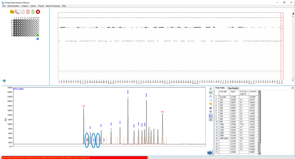
Figure 63 Main screen showing improperly fitted size calibration (too many integrated peaks, circled in blue). Solution to correct: increase the Min. Peak Height (RFU) threshold to no longer integrate extra peaks.
