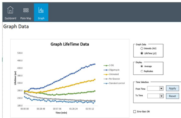
Figure 32. Graph example: pH-Xtra lifetime scale data. Average lifetime signal curves of selected samples.
