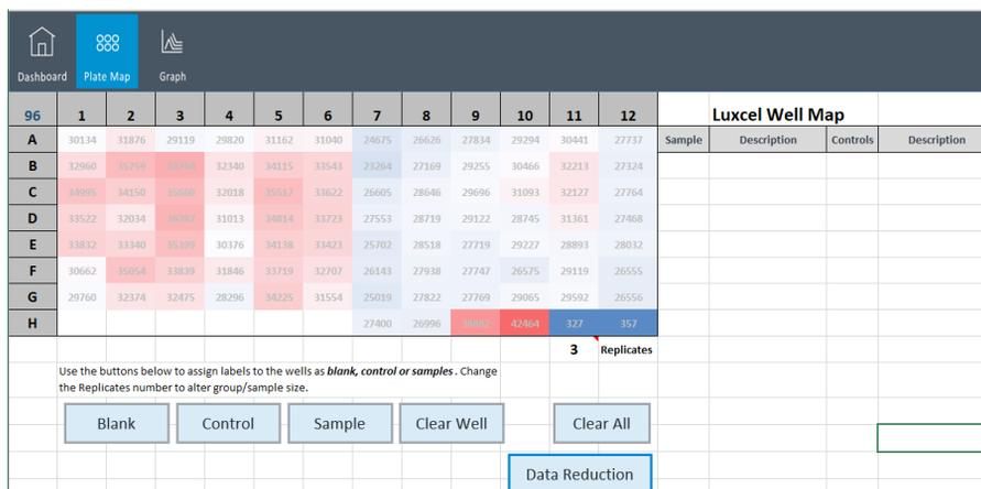
Figure 28. Plate Map Annotation; the values shown in plate map orientation are the RFU (W1) at cycle 1 of the measurement. These values are color coded based on their intensity (RFU) value, with red identifying lower AV RFU values compared to blue representing higher AV RFU value (i.e. Blank wells).
