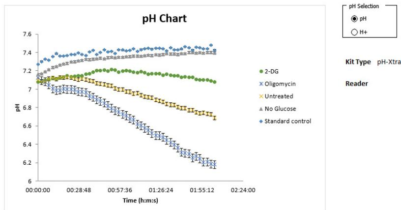
Figure 33. Graph Example: pH-Xtra pH Scale Data. Average pH scale signal curves of selected samples.
