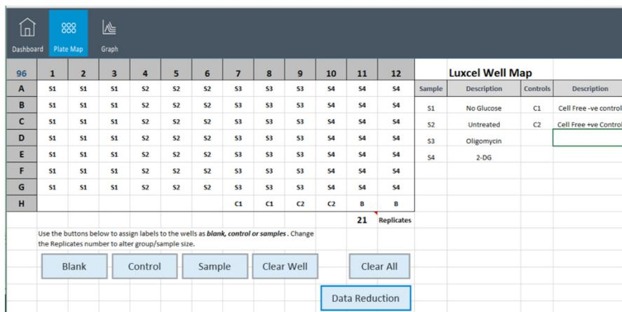
Figure 29. A completed Plate Map annotation in the Data Visualization Tool showing selected groups of Samples, Controls, and a Blank. Description information was added in the Table.
