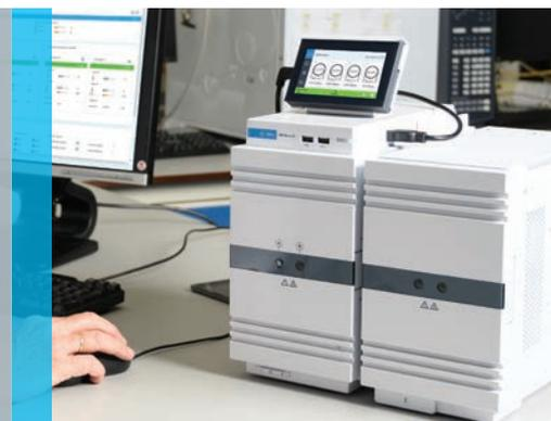
Innovative technologies deliver separate gases in seconds—in less space and with less power and carrier gas consumption than benchtop GC systems. Quick, easy startup lets you achieve results in minutes, even if you change measurement locations frequently.
