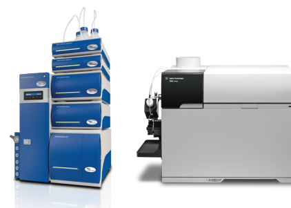
Agilent 7900 ICP-QMS coupled to PostNova AF2000MT AF4 FFF system
